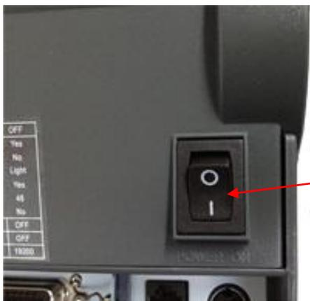
打印机电源开关
